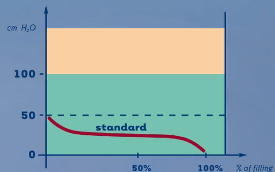
*How does system work? Redax silicone bulb permits a constant vacuum level of aspiration (around 40 cmH<sub>2</sub>O) with gradual and complete filling of reservoir in order to fully exploit its collection capacity.*
